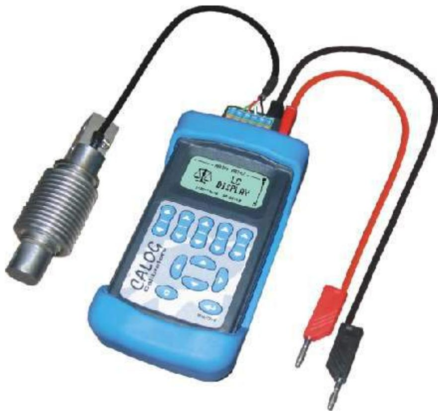
The *CALOG - LC II* is a portable, multi-function, precision instrument for strain gauge loadcell system testing and calibration. This model now includes the powerful ARM processor, a display function (ideal for portable scales or field readings), an SD card for datalogging, a USB port for connection to a computer for certificates or spreadsheets and longer lasting Lithium-Ion battery pack. Supplied complete with carrying case, charger and leads.
